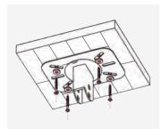
**2** Screw in the ceiling plate (4 screws and washers).
