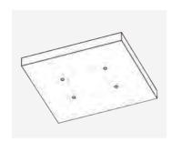
1 Use the four corner holes in the drill template to mark drill points for plugs.
