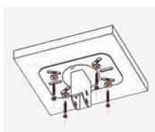
**3** Screw in the ceiling plate (2 screws and washers).
