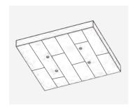
1 Use the four corner holes in the drill template to mark drill points for screws.
