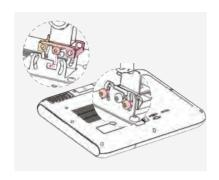
1 Take out the Obie and place middle L-shaped routings over middle screws in the tilting bracket (the Obie can be suspended in this fashion while retrieving extra screws). Retrieve the 4 hex screws and screw them in half way.
