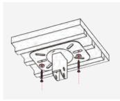
**2** Screw in the ceiling plate (2 screws and washers).
