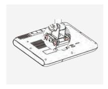
**4** Once desired projection is achieved, lock the knob and screw in the remaining four hex screws – tighten all six screws.
